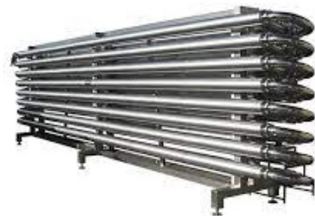
Heat Exchanger (Horizontal Tube)
